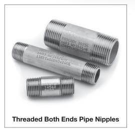
Pipe nipples are available in ASTM A403 WP316/316L or 304/304L materials, from 6 (1/8") NB upwards, threaded BSP or NPT, bevelled or plain ended.
