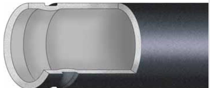
Roll groove profile (exaggerated for clarity). The small dimple created on interior pipe wall has minimal effect on pressure or flow.
