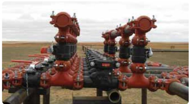
Prefabricated Well Head Assembly
