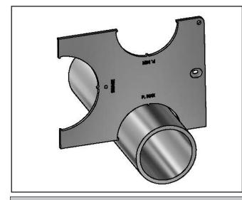
• P. Max gauge should fit 360° around the pipe. The area of the pipe to be inspected is the location where the fitting is intended to be installed.
