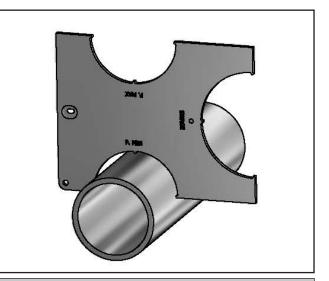
• P. Min gauge should not be able to fit at any point 360° around pipe. The area of the pipe to be inspected is the location where the fitting is intended to be installed.
