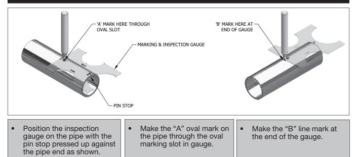
Note: The minimum space between two fittings is 2x Pipe/Tube Diameter. This allows for the inspection gauge to fit between two connections for inspection and proper operation of the fitting. It must also be noted that no fitting can be installed within the radius of a bend and only straight pipe section can be used.
