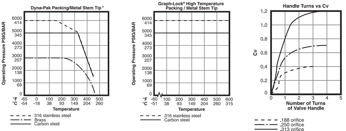
\*Curves for PCTFE stem tip are the same as above but limited to -20° to +250°F (-29° to +121 °C)
