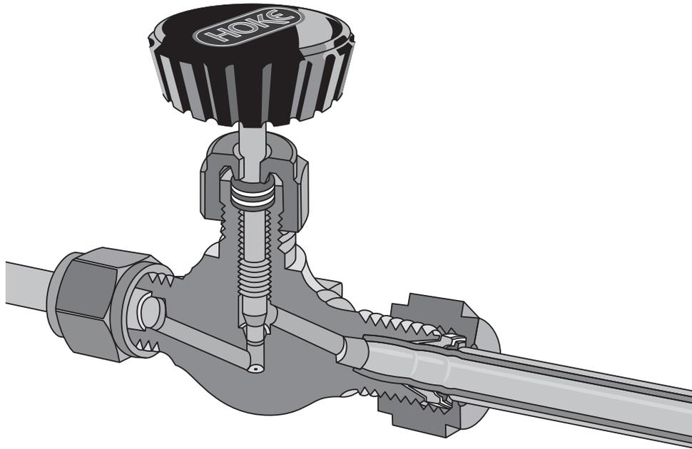
HOKE® manufactures a complete line of precision needle valves. Before making your valve selection, be sure to consider the system pressure, operating temperature, required flow and materials of construction. If your application requires a valve not available in this catalog, please contact your HOKE® stocking distributor or call HOKE® at (864) 574-7966.
