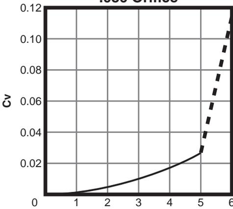
Note: Metering range of valve is within the first 5 handle turns.
