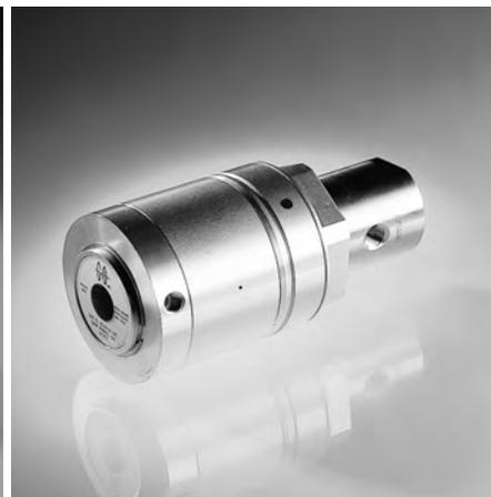
Similar in design to pressure reducing regulators, which regulate outlet pressures, back pressure regulators control the inlet pressures. Standard features allow service in many varied applications including corrosive fluids and with the optional features available, the user can tailor these units to suit virtually any application.
