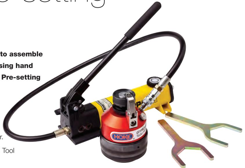
Using the portable Hydraulic Pre-setting Tool, the GYROLOK® nut and ferrule system is initially set onto the tubing. The pre-set fitting and tube assembly is then easily installed by following the GYROLOK® reassembly instructions.
