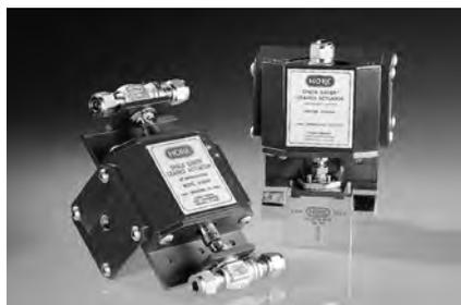
Select HOKE® valves can be remotely actuated. Pneumatic or electric operators provide flexibility and convenience. HOKE® pneumatic actuators feature a unique space saving concept and the ability to operate two valves on the same actuator (pictured). Electric actuators are offered both as weather-proof or explosion-proof units in 115 Volt AC or 24 Volt DC versions.
