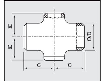
The function of a cross is similar to that of a tee with the exception of providing two 90° outlets opposite each other. Equal crosses have all four outlets of equal size. Reducing crosses have branches that are smaller in size to that of the run to obtain the desired flow and pressure through the system.
