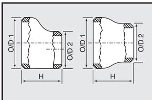
The function of both types of reducer is to reduce the line from a larger to a smaller pipe size, this obviously results in an increased flow pressure. With the eccentric reducer the smaller outlet end is off centre to the larger end enabling it to line up with one side of the inlet and not with the other.
