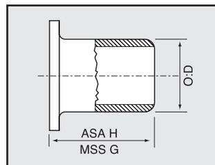
A stub end and its associated slip-on flange allows quick disconnection of the particular section involved as well as easy alignment of mating flanges. Stub ends are installed in pairs and mated together with two slip-on flanges.
