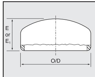
The function of an end cap is to block off the end of a line in piping systems. This is achieved by placing the end cap over the open line and welding around the joint.
