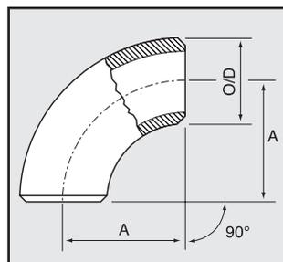
The function of a 90° elbow is to change direction or flow in a piping system.
