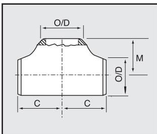
The function of a tee is to permit flow at 90° to the main direction of flow. The main flow passes through the 'run' whilst the 90° outlet is known as the 'branch'. The equal tee is manufactured with all three outlets being the same size.
