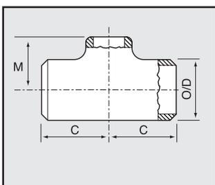
The reducing tee is manufactured with the branch outlet smaller than the run to obtain the desired flow and pressure through the system.
