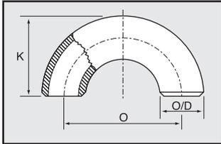
The function of a 180° return bend is to change direction of flow through 180° and there are two basic types, long radius and short radius. Both types have a centre to centre dimension double the matching 90° elbows. The primary application for these fittings is in heater coils and heat exchangers, boilers etc.
