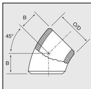
The function of a 45° elbow is the same as a 90° elbow, but the measurement of dimensions, however, is different to that of the 90° elbow. The radius of a 45° elbow is the same as the radius of the 90° LR elbow where 'R' equals 1-1/2 x D. However, the centre to face
