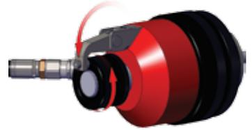
Pump the handle until the indicator arm releases.
