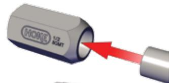
Mark the tubing as shown with an Ultra-Fine Point, Chloride-Free pen (recommended Sharpie Model 37001). Take care to position the marker perpendicular to the GMT, or insufficient ferrule set could occur.
