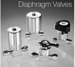
The DV Series Diaphragm Valves are totally free of springs, bellows, packing, o-rings and lubricants in the process wetted area. Metal to metal seals to atmosphere ensure that there is no absorption of undesirable elements into the flow stream. Elgiloy® diaphragms ensure the utmost in corrosion resistance and life span.
