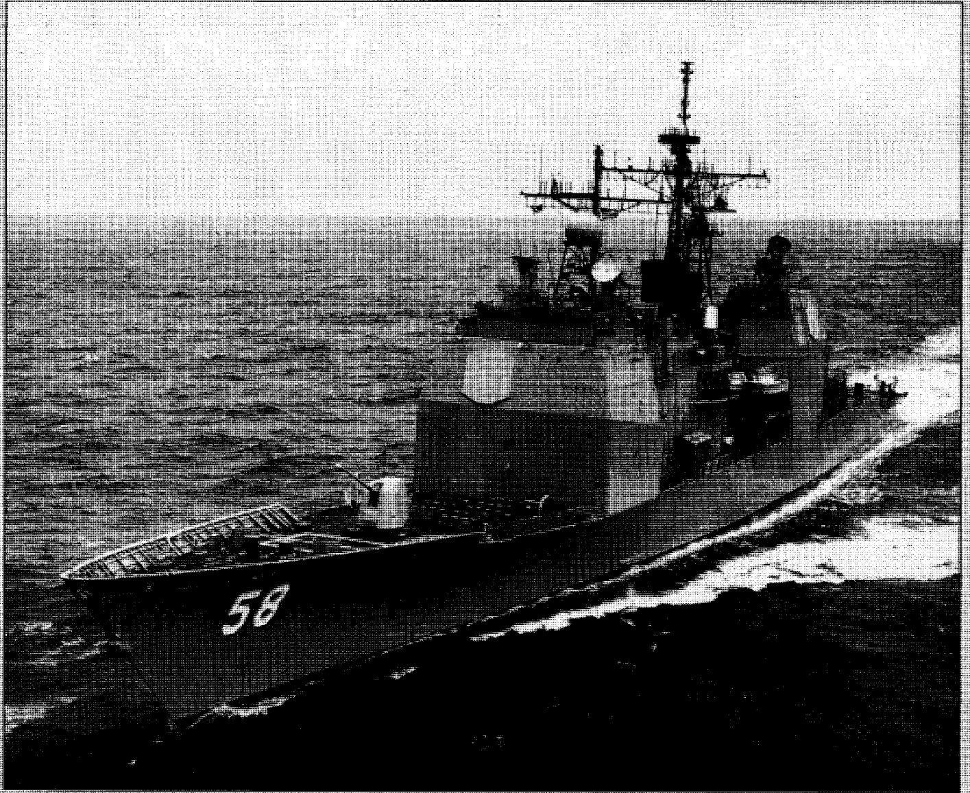
U. S. Naval vessel Philippine Sea , Aegis missile cruiser constructed Bath Iron Works, Maine, LOA 173' (56.7m), beam 55' (15.76m), 9468 tons full-load. Four gas turbines generate 80,000 shaft horse power. Range 6,000 nautical miles, complement 385.
