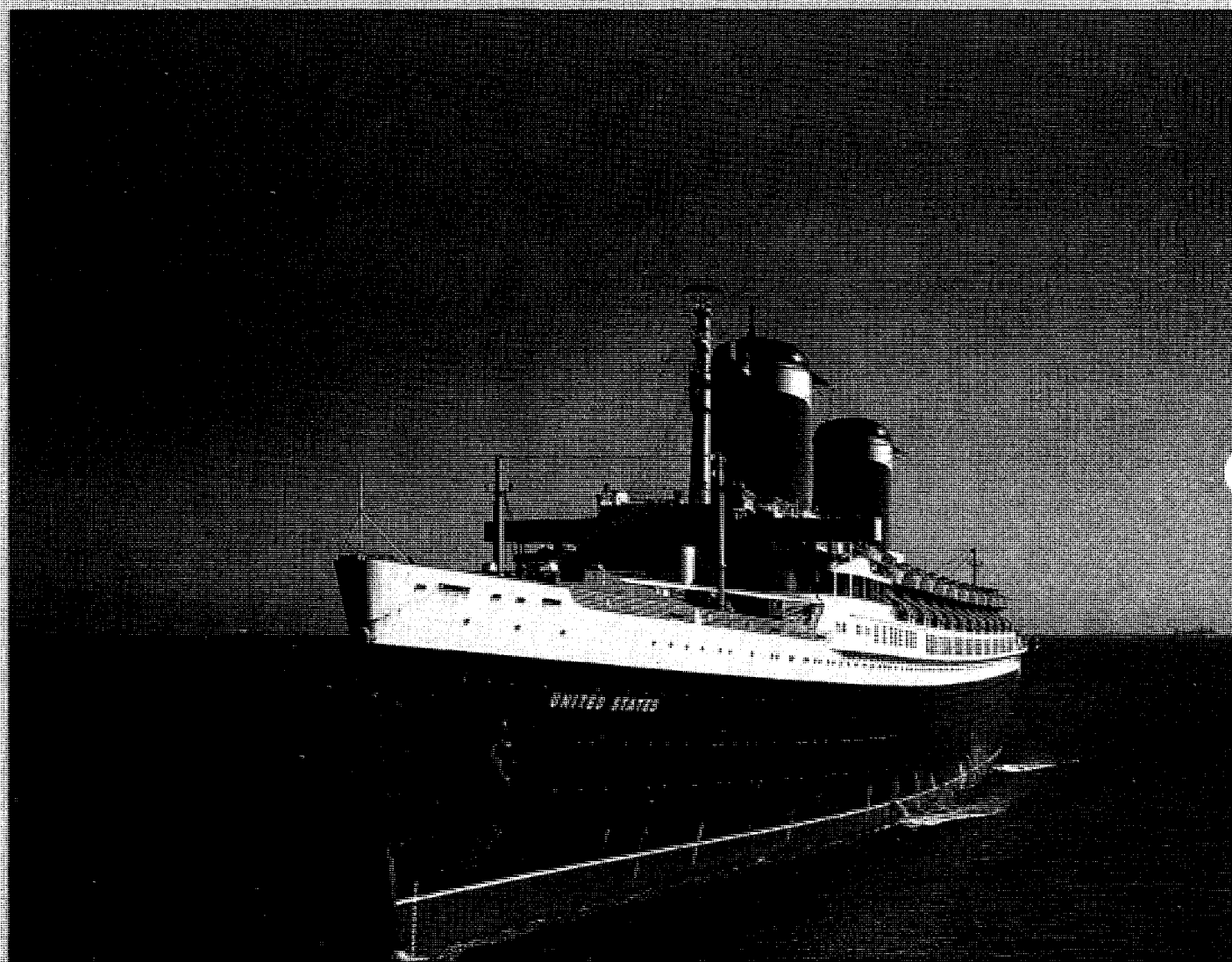
S.S. United States built 1951-52 at Newport News Shipbuilding and Drydock as Hull 488, with an aluminum superstructure. Length 989.7' (301.7m), beam 101.5' (31m), draft 32' (9.8m), gross tonnage 38216.8 steam turbines generate 173800 shaft horsepower. Taken out of service 1969. At this printing, owned by a Turkish concern and in Russia for asbestos removal.
