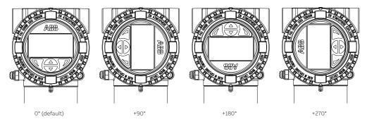
**5** Push back the display module on the communication board, making sure that the four plastic locks are properly fixed.
