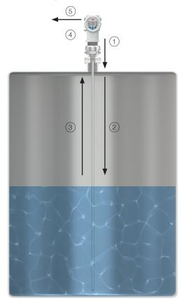
The head sends a very short pulse of microwave energy through the coupler and down the probe (1). That pulse travels along the length of the probe (2) and, when it encounters the product surface, some of the energy is reflected and travels back towards the coupler (3). When the reflected energy reaches the coupler, it is sensed by the electronics (4). By measuring the time elapsed between the initial pulse and the reflected one, the electronics can calculate the product level (5).
