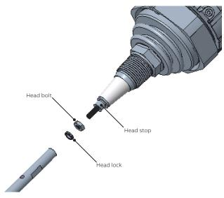
**3** Screw in the probe end and tighten by hand.
