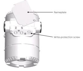
**2** Using a suitable screwdriver, fully press down on the write-protection screw and turn 90° clockwise to activate hardware write protection or, if already activated, 90° counterclockwise to deactivate it.
