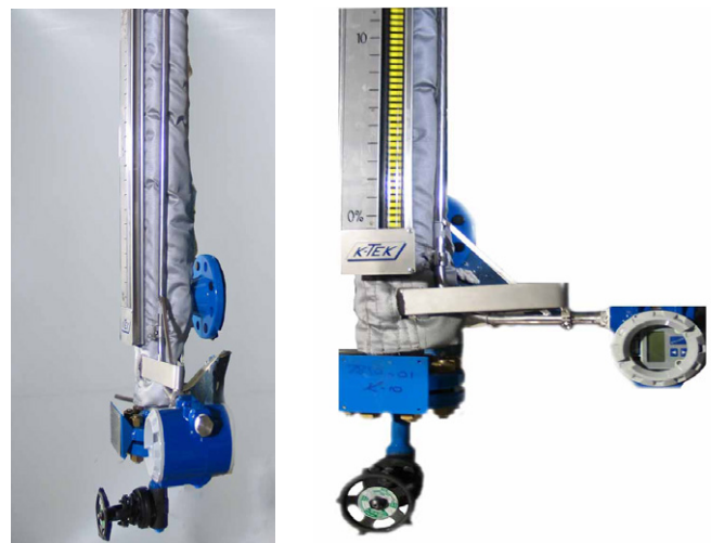
Figure 22 - side and front view of pipe wrap
